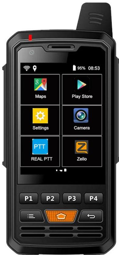
The FleetWave-LTE FWH-F50 Push-to-Talk over Cell radio provides instant and reliable communication at the push of a button. The FWH-F50 utilizes 4G LTE data to provide nationwide coverage suitable for all kinds of industries such as construction, transportation, fire and rescue, and many more.
